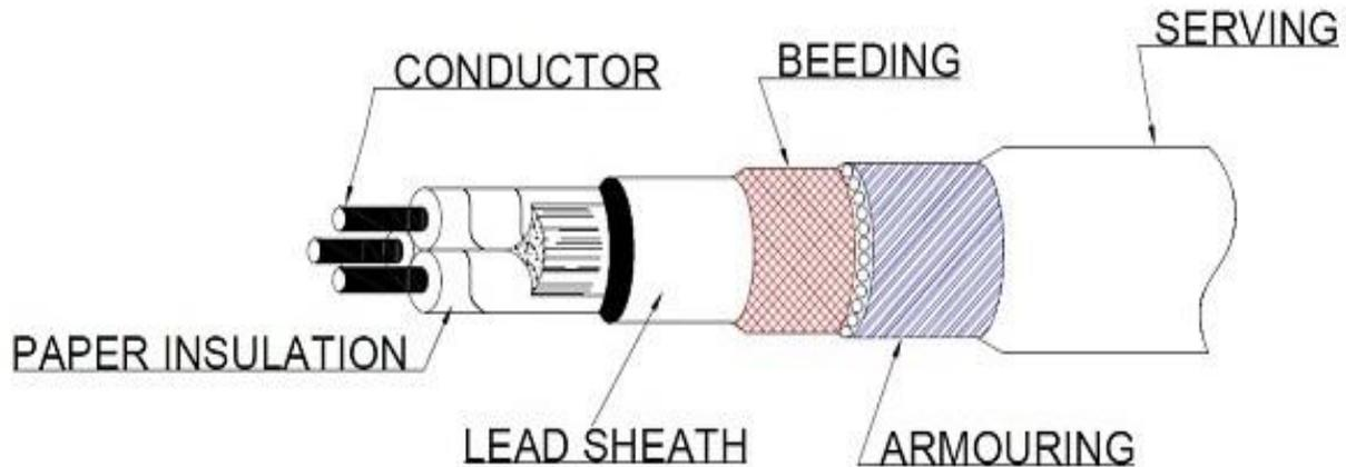
**Metallic sheath:** In order to protect the cable from moisture, gases or other damaging liquids (acids or alkalis) in the soil and atmosphere, a metallic sheath of lead or aluminium is provided over the insulation as shown in Fig.
